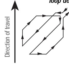
right edge of the loop is often sensitive enough to detect bikes and can be marked with a special pavement marking. A number of cities have experimented with various designs; the San Diego design is shown below.
