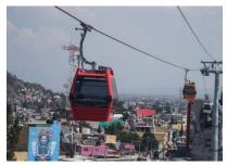
tramways, these systems are a type of cable car pioneered for ski resorts, but have been deployed in urbanized areas to avoid the issues related to surface infrastructure. Passenger capacity can range from four passengers up to 100 per car, and the systems will typically have only two cars and two stops.
