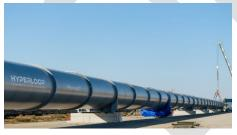
system that uses evacuated tubes to move multipassenger vehicles at speeds up to 700 mph. Several companies are currently developing prototypes, and planning has been started to deploy the systems in routes in several key markets within the U.S.
