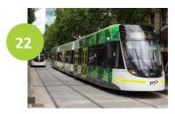
**Tram / Trolley / Streetcar** – Typically an electric railway with a "light volume" traffic capacity compared to heavier rail. The system may use shared or exclusive ROW, high or low platform loading, and multi-car trains or single cars, and are not compatible with freight rail.
