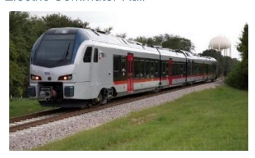
Passenger rail service operating on fixed rails typically providing an interurban or regional service. Commuter rail typically has a higher volume ridership capacity and relatively longer distance between stops compared to light rail. Operations on a single track with sidings allows for two-way travel.
