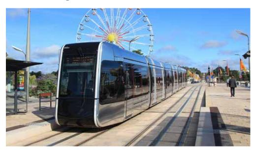
Passenger rail service operating on fixed rails typically providing an urban or interurban service with a lighter volume ridership capacity compared to commuter rail. Operations on a single track with sidings that allow for two-way travel.
