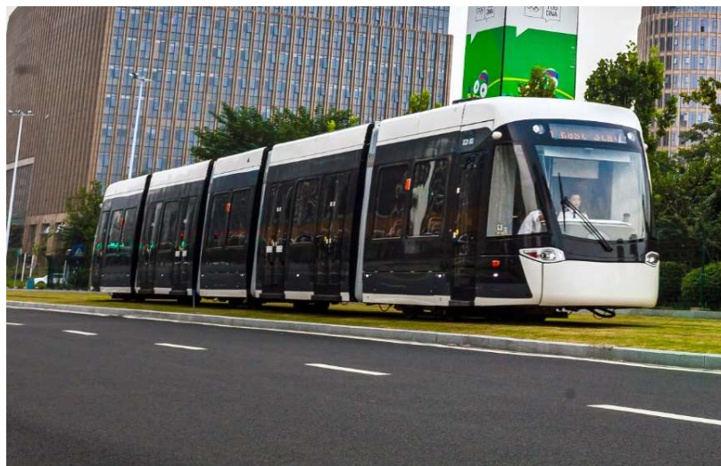
Figure 2.5: Bombardier Flexity - battery electric train with MITRAC batteries allows 100km catenary free propulsion. https://rail.bombardier.com/en/solutions-and-technologies/urban/e-mobility-battery-technology.html
