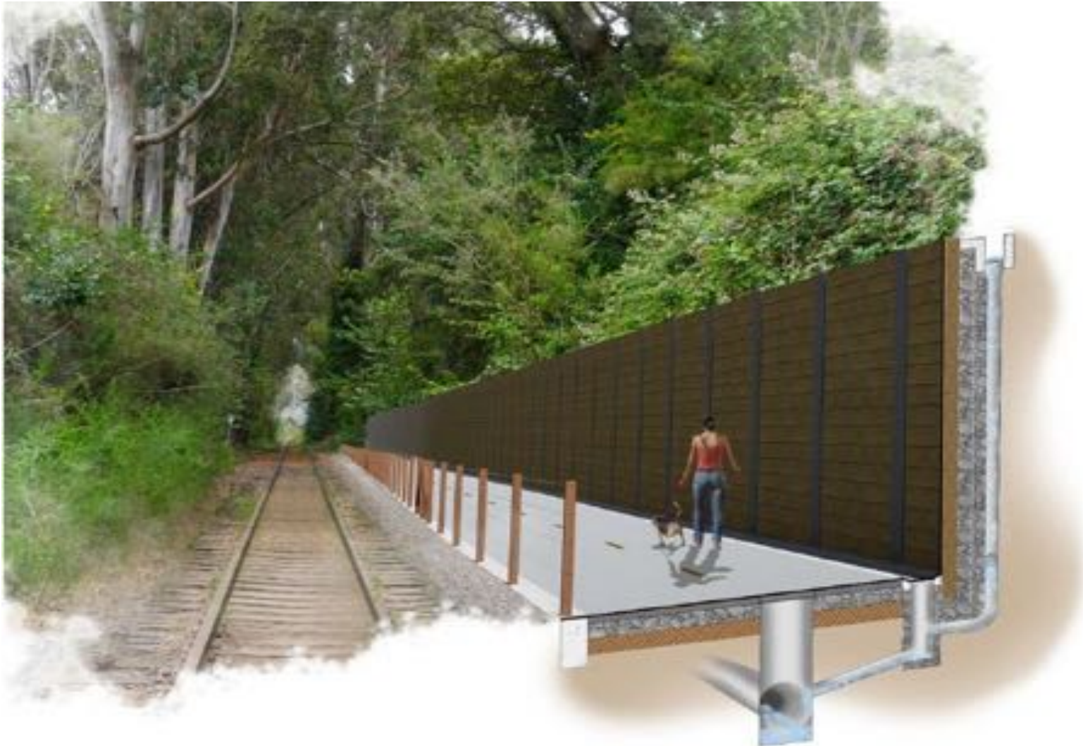
Depot Hill retaining wall and storm drain solution.
