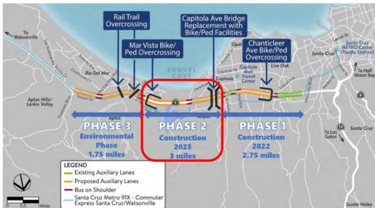
Figure 1 - Phase 2 Project includes 3 miles of auxiliary lanes and bus on shoulder improvements in both directions of Highway 1 between the Bay/Porter and State Park Drive interchanges, retaining walls, soundwalls, replacement of the Capitola Avenue Overcrossing, and a new bicycle/pedestrian overcrossing at Mar Vista Drive
